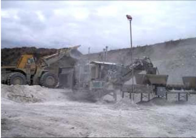
A Caterpillar loader dumping 22 tons of rock into the crusher
